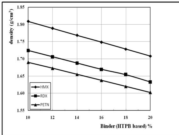
Figure.1 Effect of binder percentage (based on HTPB) on the density of PBX formulations
