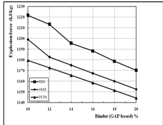
Figure.8 Effect of binder percentage (based on GAP) on the explosion force of PBX formulations
