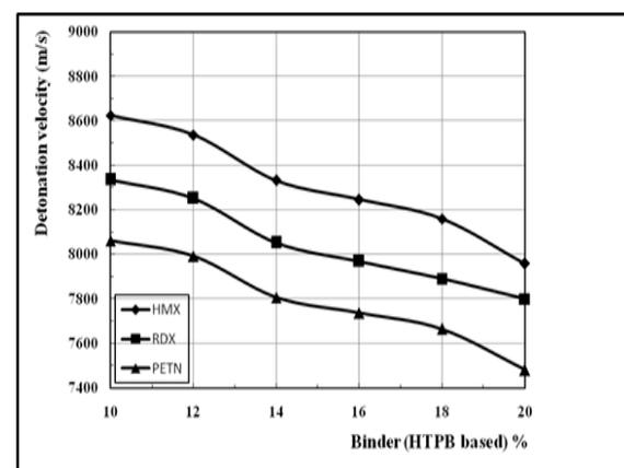
Figure.4 Effect of binder percentage (based on HTPB) on the detonation velocity of PBX formulations
