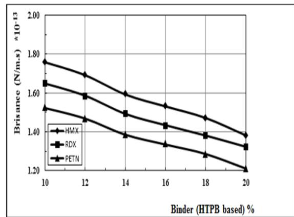
Figure.10 Effect of binder percentage (based on HTPB) on the brisance of PBX formulations
