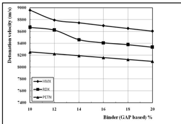
Figure.5. Effect of binder percentage (based on GAP) on the detonation velocity of PBX formulations
