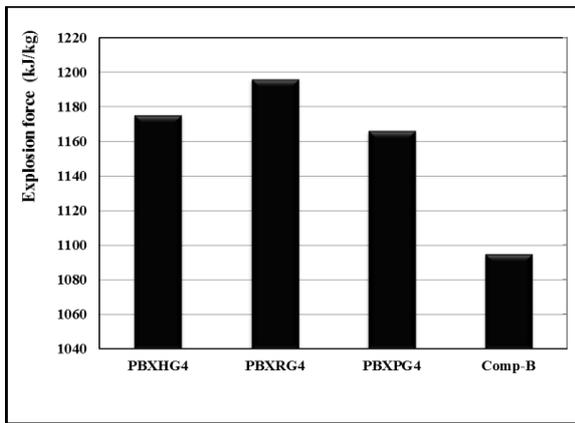
Figure.9 The explosion force of PBX formulations based on 14% PU (based on GAP) and comp-B
