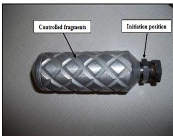
**Figure 13.** Photograph of the used controlled fragmentation testing cylinder casing.
