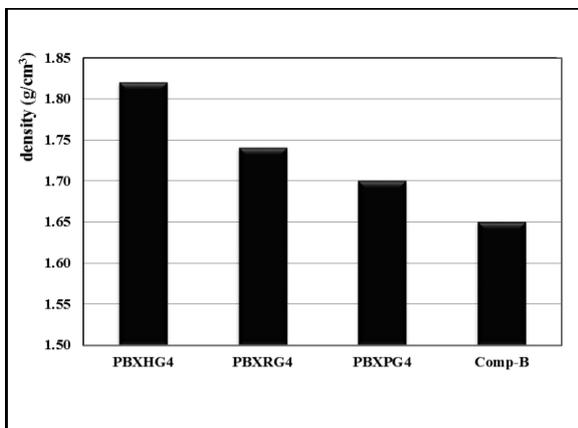
Figure.3 The density of PBX formulations based on 14% PU (based on GAP) and comp-B
