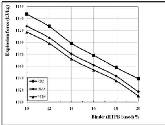
Figure.7 Effect of binder percentage (based on HTPB) on the explosion force of PBX formulations
