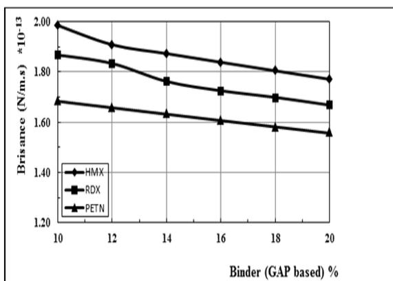
Figure.11 Effect of binder percentage (based on GAP) on the brisance of PBX formulations
