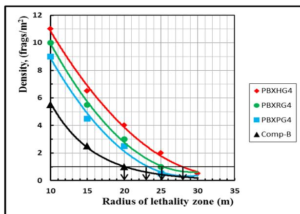
**Figure 14.** Warhead lethality zone of the warhead filled with comp-B and PBX formulations based on GAP.
