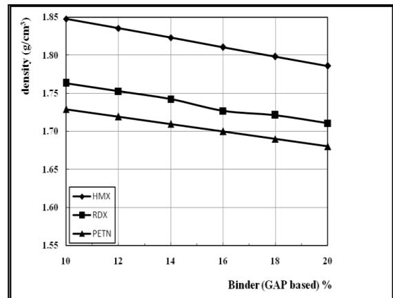
Figure.2 Effect of binder percentage (based on GAP) on the density of PBX formulations
