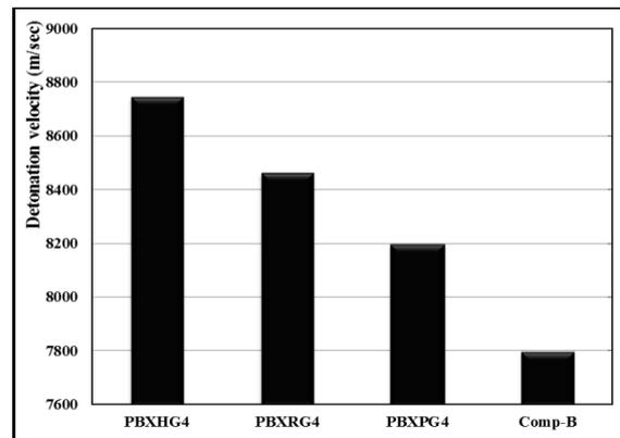
Figure.6 The detonation velocity of PBX formulations based on 14% PU (based on GAP) and comp-B
