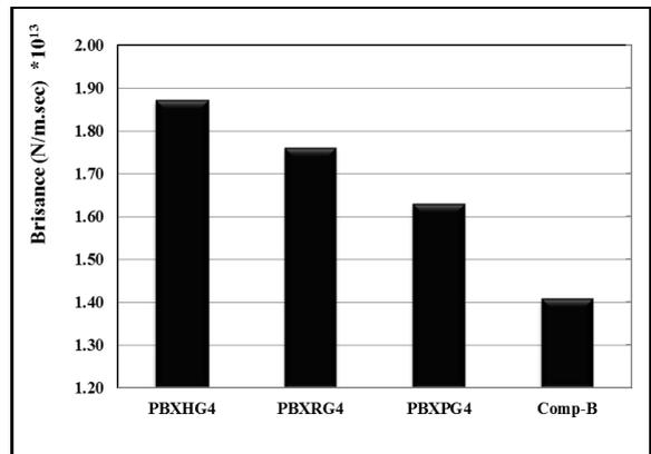
Figure.12 The brisance of PBX formulations based on 14% PU (based on GAP) and comp-B
